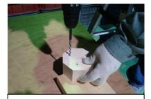
(5) Drill pilot holes the same diameter of the screws so that the wood base does not crack.
