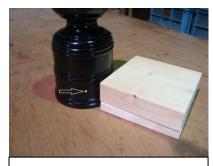
① Check the height of the screw holes on the Giboshi itself to determine the thickness of the wood base.
