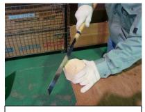
④ Use a saw to cut the wood base on the lines of the octagon drawn.
