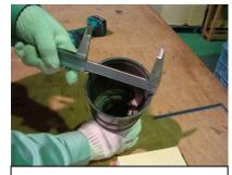
② Measure the internal diameter of the Giboshi so that it can be marked on the wood base.
