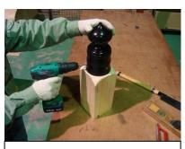
Screw the Giboshi to the wood base. Tighten each screw equally.
