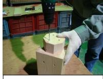
6 Attach the wood base to the column with screws long enough to reach through the wood base into the column.
