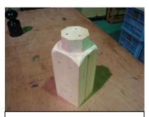
⑦ Chamfer the corners of the column so that water does not collect.
